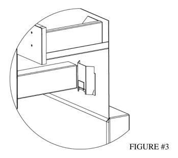
When heating with steam, the supply connection should be attached to the uppermost tube and the return to the lower tube. The coil is pitched in the casing to allow drainage of condensate.
