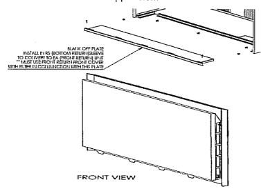
Note that an ACCEA\_RSRETROFIT\_SIMPLE is also available — it is a less costly RETROFIT Kit utilizing the simple single panel cover but with less sound suppression.
