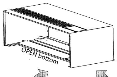
The OPEN Bottom sleeves (open on the first 6" of the sleeve facing the room) were made by McQuay, Singer, Remington to provide bottom-return airflow for the original RS Heatpump designs.
