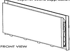
ACCEA\_FTCOVER\_SIMPLE -- simple single panel design with grille cuts directly on front panel as shown, with less sound supression, but at a lower cost.
