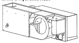
Applied Comfort's EA is designed to function with the original EA front covers (McQuay, Singer, Remington) with air return around the entire periphery of the front cover. We also offers 2 optional covers:
