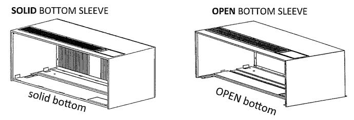
When installing EA, RS, and ES replacements, ensuring proper evaporator airflow is critical.
