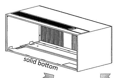
EA, RS, and ES chassis can be installed into original SOLID BOTTOM sleeves, if the correct front covers are used. The Solid Bottom sleeves were the dominant type made by McQuay, Singer, Remington – solid except for a hole for power cords.
