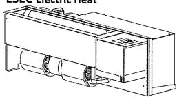
RS and ES chassis can be installed directly into original OPEN BOTTOM sleeves with original covers. The following replacement cover is also available.
